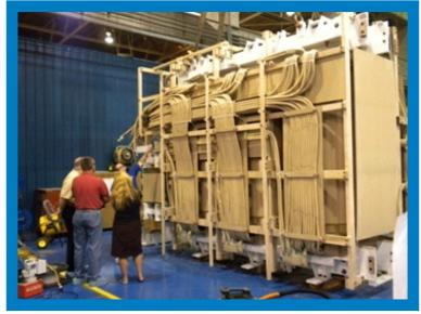
Weather is holding up the construction of the New Substation but it isn't holding up construction of its heart which is the 138,000/12,000KV transformer being built in Pocatello Idaho by Virginia Transformer. Here is a picture of our engineering consultants Norm Baron and Jim Havrilla of Utility Engineers inspecting the core and coils. Delivery of the substation has been pushed back to June or July.
